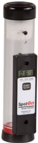
Spot-On sprayer calibrator model SC-1 Innoquest, Inc.; Woodstock, IL
