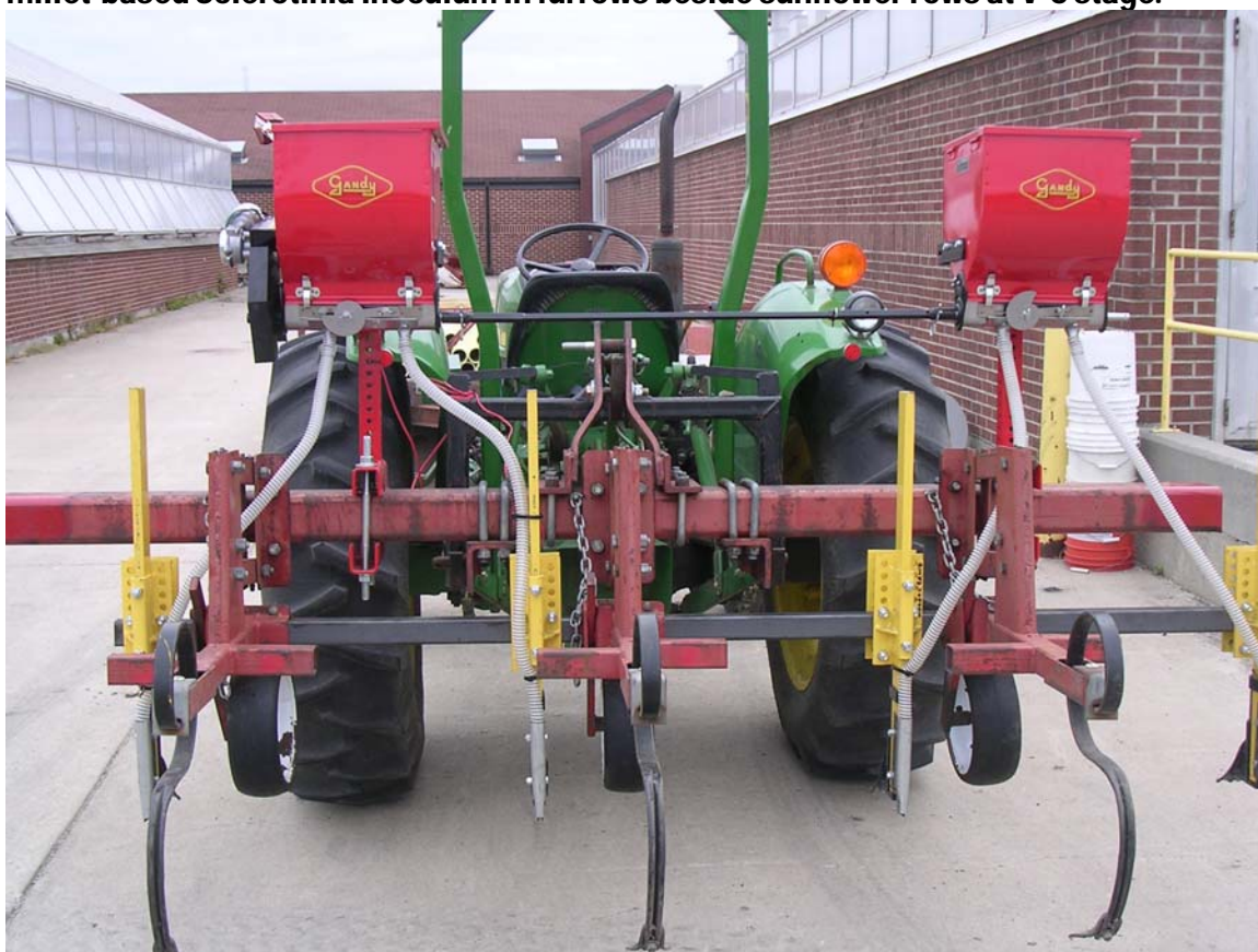
Figure 1. Granular chemical applicator mounted with anhydrous ammonia shanks used to deliver millet-based Sclerotinia inoculum in furrows beside sunflower rows at V-6 stage.
