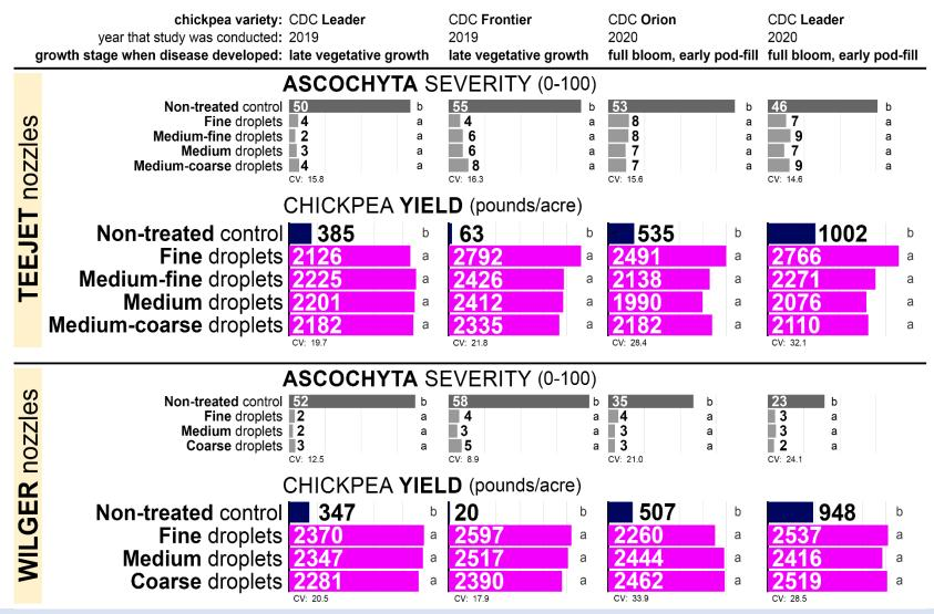
Wilger Combo-Jet flat-fan nozzles. FINE DROPLETS: ER110-04, 50 psi (2019); ER110-05, 60 psi (2020); MEDIUM: SR110-04, 50 psi (2019); SR110-05, 60 psi (2020); COARSE: MR110-04, 50 psi (2019); MR110-05, 60 psi (2020). TeeJet XR flat-fan nozzles. FINE: XR11004, 50 psi (2019), XR11005, 60 psi (2020); MEDIUM-FINE: XR11005, 40 psi (2019), XR11006, 50 psi (2020); MEDIUM-COARSE: XR11008, 40 psi (2019, 2020). Spray volume: 15 gal/ac Driving speed: 8.9 mph (2019), 10.5 mph (2020)
