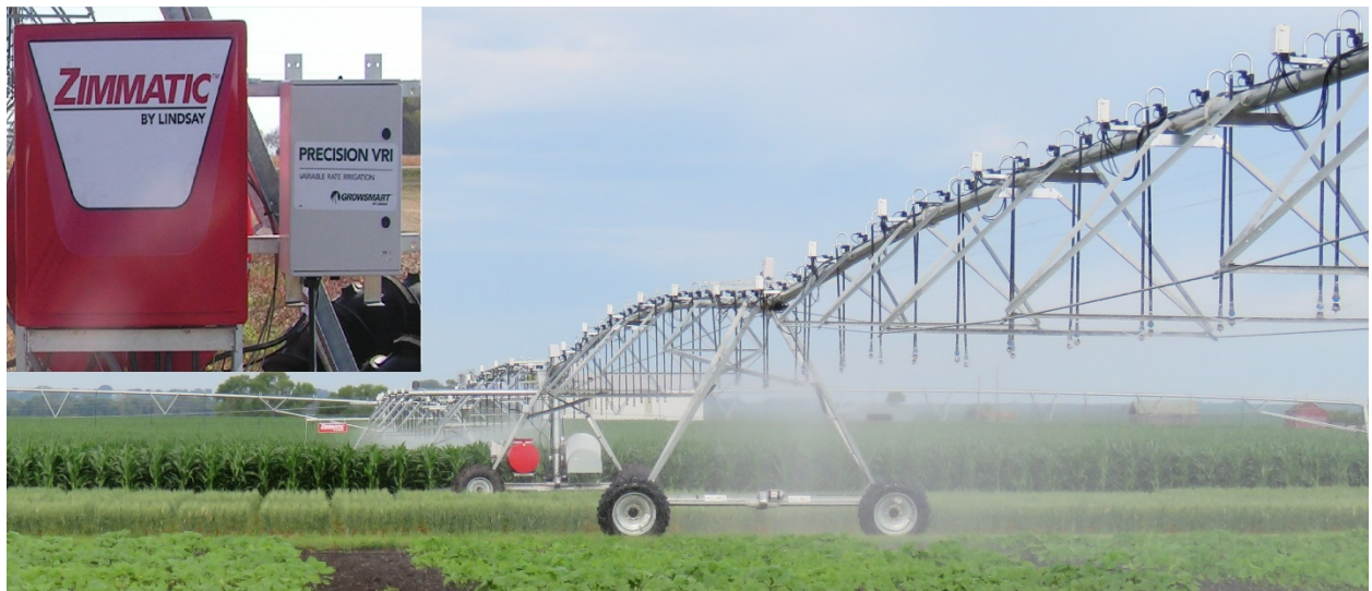
Figure 2. Our new Lateral with Variable Rate Irrigation capability.
