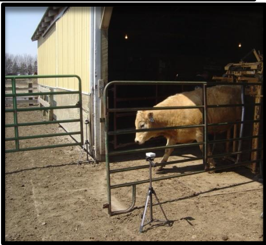
Figure 1A) Exit velocity setup. The “start” sensors were placed three feet from the head gate and the “finish” sensors set 6 feet away. B) Exit velocity was recorded as the time for the steer to run 6 feet from the exit of the working chute.
