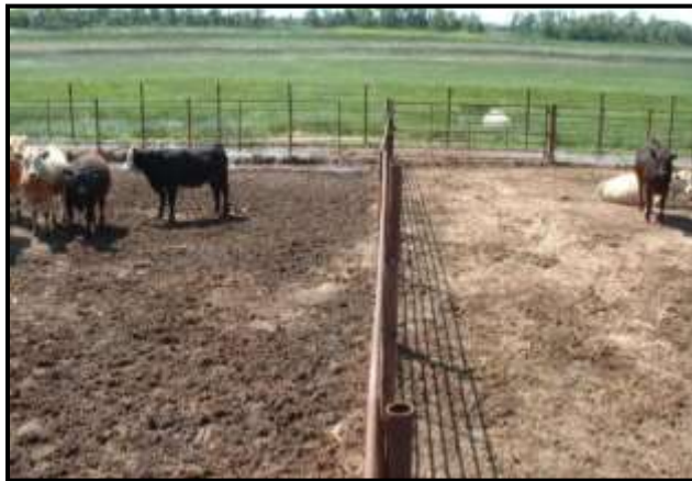
Photo 2. Fly ash, right, versus control pen (left) surfaces, three years after placement following a two-week summer rainfall period.
