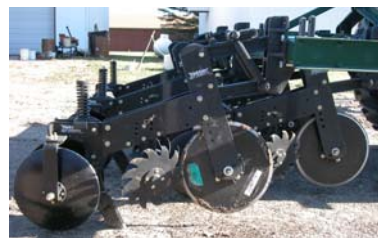
Figure 1. Yetter strip-till unit used in trial.
