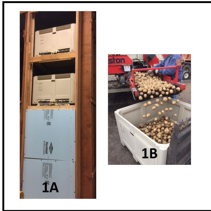
Figure 1. One of three pressure towers located at the USDA-ARS facility (EGF, MN) (1A). Foam insulation is removed from the top shelves for picture clarity. Air flow is directed through the tote from a 3" duct located at the back wall (not shown). The front forklift holes are filled to ensure humidified air is uniformly directed through the tote (1.5 cfm/cwt). A chip variety collected from a cooperated clod hopper at Hoople, ND (1B).
