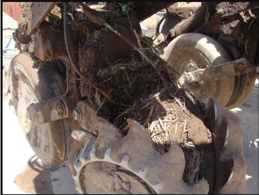
Figure 5. Row cleaners and press wheels are key areas that accumulate unintended biomaterial/soils.
