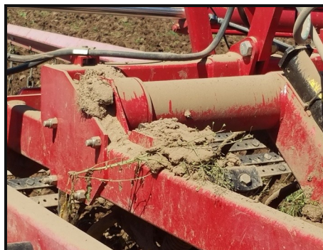
Figure 3. Remove as much plant and soil material as you reasonably can to limit unintended transport.
