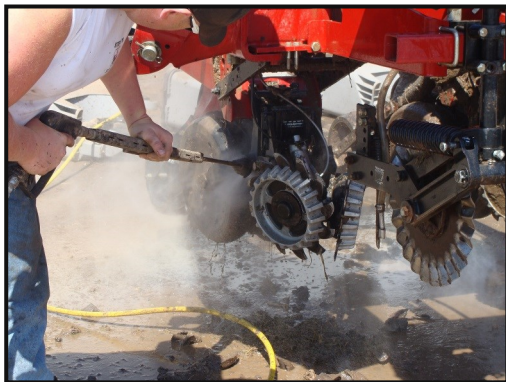
Figure 6. It took approximately one hour to remove the biomaterial/soil from this 12-unit planter to prevent...
