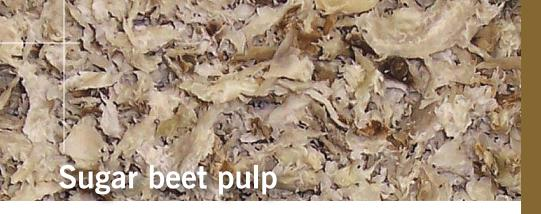
Preliminary research is being conducted into the use of sugar beet pulp as a feedstock for ethanol production. This feedstock has potential because it hydrolyzes (breaks down) without the use of harsh thermochemical pretreatments that are required for perennial grasses and other biomass feedstocks, according to NDSU scientist Scott Pryor.
