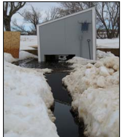
Spring 2009 snowmelt provides ample opportunity for runoff monitoring. Pictured is one of three gaging stations at Johannes Farm and Feedlot.
