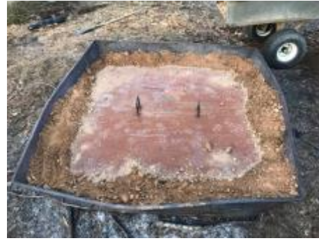
Figure 9. When the Flame Cap Kiln is full of glowing coals, it is time to quench it. Flood quenching is most effective, but dry quenching can also be used. Here (above) a thin sheet steel lid is placed on top of the hot coals and sealed with dirt or clay. Photos: WBA
