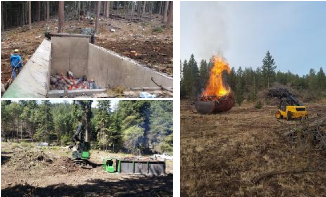
Figure 11. Left: An Air Curtain Burner designed for complete incineration is able to make biochar if the air is controlled properly. This unit operating on the Rogue-Siskiyou National Forest made 20 cubic yards of biochar (Photos: WBA). Right: arborist Brandon Baron makes biochar in a modified 10,000-gallon water tank (Photo: The Tree Service, Burns, Oregon).
