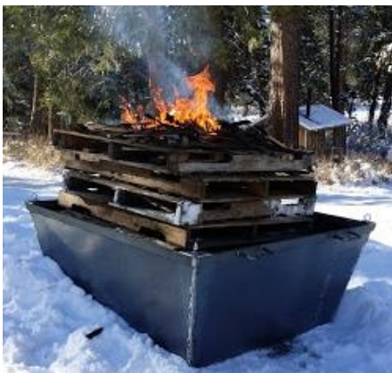
Figure 8. The Oregon Kiln making biochar on a small goat dairy for use in the barn. Start the Flame Cap Kiln with a top-lit rick. Once the initial charge burns down, start adding new material in layers. The flame front moves down as the rick burns down, and then moves back up as the container is filled. Photos: WBA
