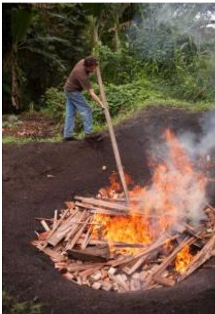
Figure 10. Left: A pit kiln used in Hawaii to produce commercial quantities of biochar (photo: Josiah Hunt, Pacific Biochar). Above: a cone-shaped kiln available from the Moki company chars bamboo in Japan.
