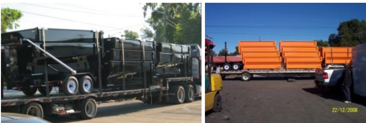
Figure 14. Left: Nesting 12-yard dumpster with roll-off trailer transported on lowboy. Right: Nested 20-yard dumpsters.
