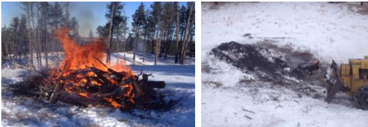
Figure 13. Snow quenching in Nebraska. Rowdy Yeatts of High Plains Biochar uses snow to quench Conservation Burn piles.
