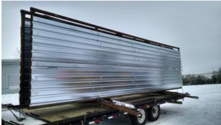
Figure 16. Cattle panel windbreaks can be deployed as a "Burn Corral" to improve burning efficiency of a pile.
