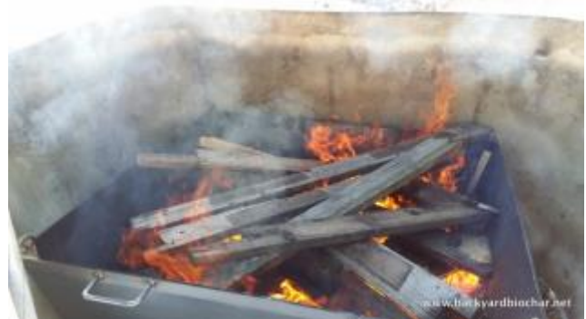
Figure 8. The Oregon Kiln making biochar on a small goat dairy for use in the barn. Start the Flame Cap Kiln with a top-lit rick. Once the initial charge burns down, start adding new material in layers. The flame front moves down as the rick burns down, and then moves back up as the container is filled. Photos: WBA
