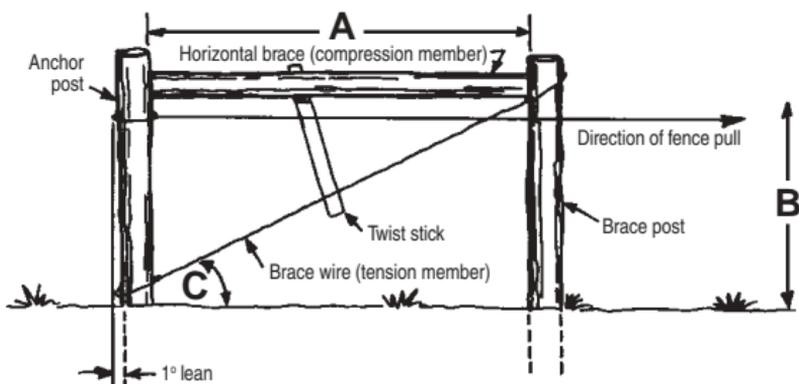
poor corners generally require more maintenance and have a shorter life span than those with well designed and installed corner braces.
