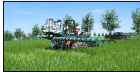
Figure 2. Air assist sprayers push the grain heads forward to help improve coverage when applying fungicides.
