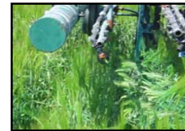
Figure 4. Air velocity changes the orientation of the head improving fungicide coverage.
