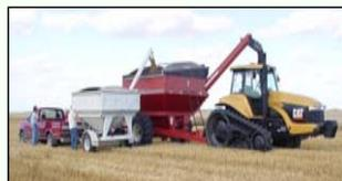
**Figure 2.** MN grower using his tractor, grain cart, and combine to assist with research during harvest. One combine swath from each plot was made. Grain was transferred to the weigh wagon (white) and yield was determined.
