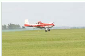
Figure 1. Cessna Ag Truck aircraft with CP-03 nozzles used by a commercial North Dakota aerial applicator for fungicide application on spring wheat in ND and MN, 2005.
