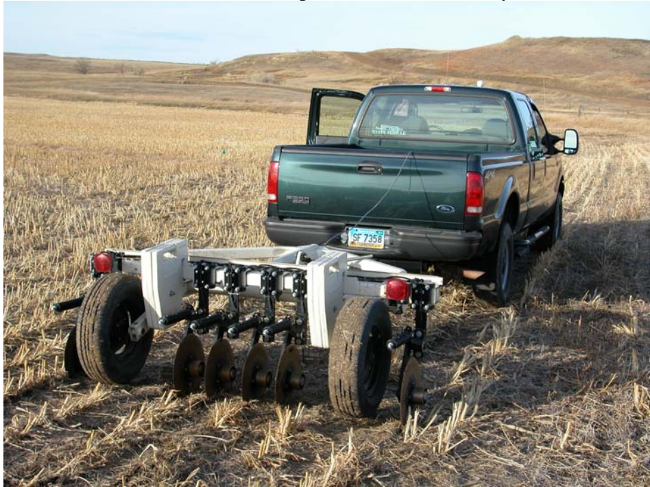
Figure 4. Veris 3100 machine used to map electrical conductivity of the soil.
