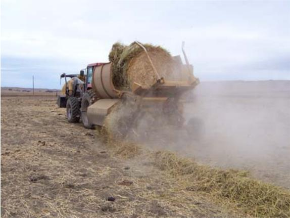
**Figure 4. Tapered-Cone Bale Feeder.**
