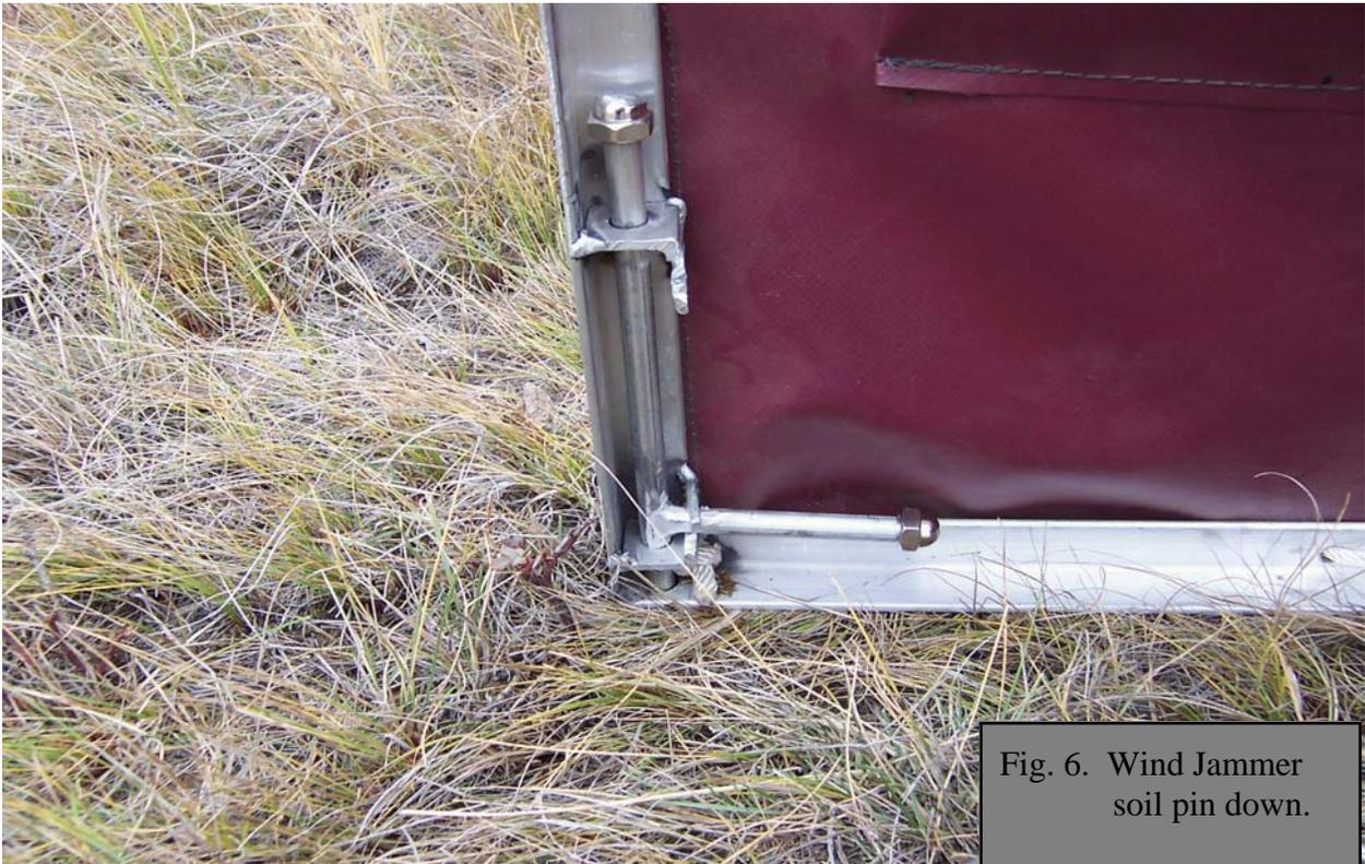
Fig. 6. Wind Jammer soil pin down.
