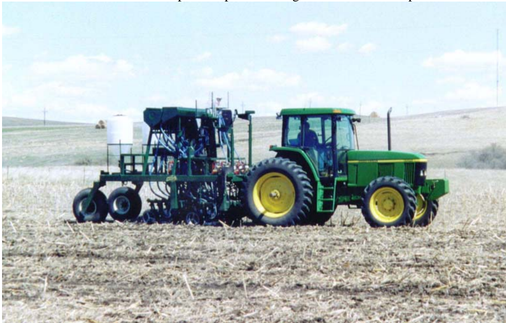
Figure 3. The DREC Cross-Slot™ opener no-till plot drill seeding field pea in corn residue at Center, ND, 2004. This drill can seed both small replicated plots and large demonstration strips.
