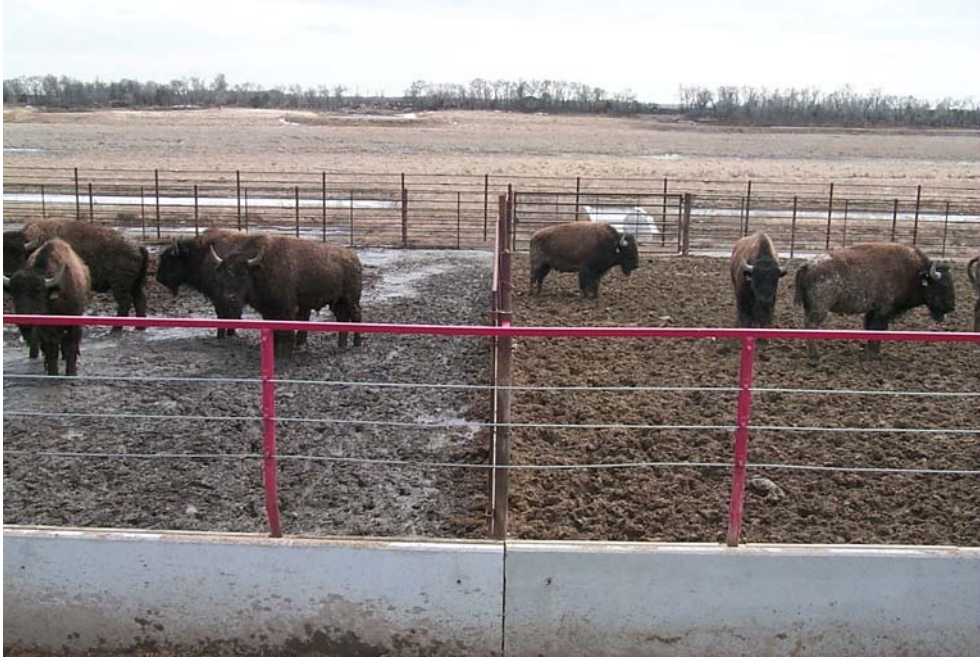
Pen B5, left, is a control pen containing no coal ash. Pen B4, right, contains 25% coal ash. Based on visual results, soil in the treated pen appears to perform much better than soil in the untreated pen.
