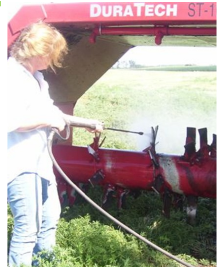
Initial power-washing of a compost turner. Photo courtesy of Anne Ehni, Wells County SCD Manager.
