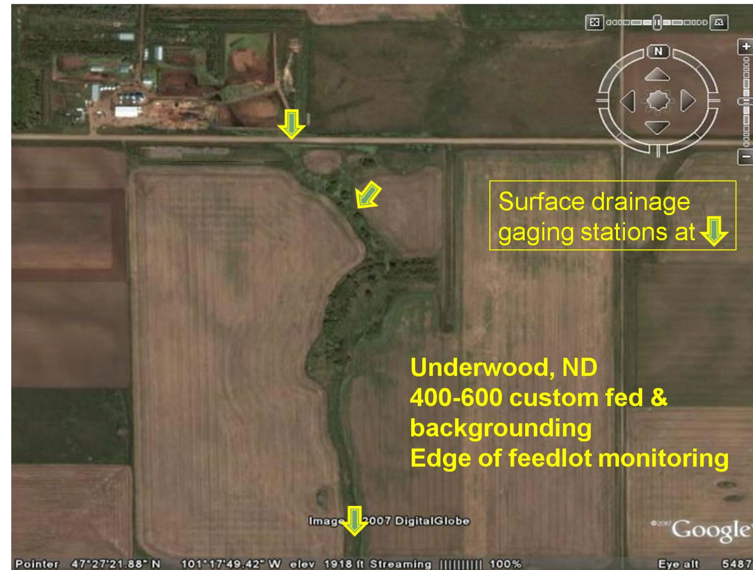
Figure 1. Aerial photo of feedlot and field surface runoff monitoring stations at location 1 in Underwood, ND.
