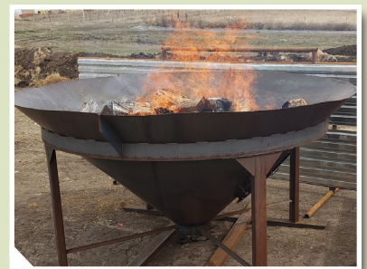
Converting wood into biochar in a kiln fabricated from a hopper bin bottom. Photo Credit: Kelpie Wilson
