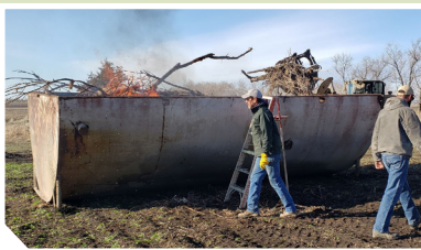
Loading trees and branches with a wheel loader into an oil tank biochar kiln. Photo Credit: Kelpie Wilson
