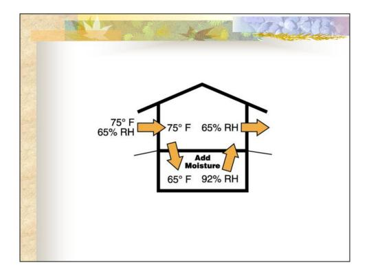
During the summer, ventilation may increase the moisture in a basement where it is cooler than outdoor temperatures. Cooling air decreases it's moisture holding ability and increases it's relative humidity. Air at 75° F and 65% relative humidity will have a relative humidity of 92% when cooled to 65° F in a cool basement. Therefore, moisture should be removed by running a dehumidifier or an air conditioner.
