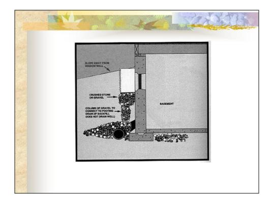
There should also be a granular connection from the window well to the drain tile to assure drainage away from basement windows. Place a layer of crushed stone or gravel under the window well to aid in drainage. Keep leaves and other debris from clogging the crushed stone.
