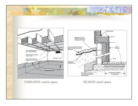
Crawl spaces need moisture control similar to that used in a basement to keep the soil in the crawl space dry. There should be a vapor retarder covering the floor of the crawl space that is bonded to the footing wall. A vent should be available to remove moisture if it accumulates in the crawl space. The vent is normally closed to keep moisture from the outdoor air entering the crawl space.
