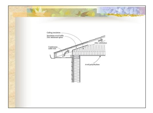
The potential for ice dams can be reduced by putting more insulation in the ceiling, providing soffit venting into the attic, and blocking any airflow paths from the living space into the attic.
