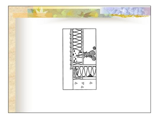
All openings in the wall, such as around electrical outlets, or ceiling, such as around recessed light fixtures, need to be sealed to limit moisture transfer into the wall or ceiling. Large amounts of moisture can be transferred through an opening in the wall or ceiling.
