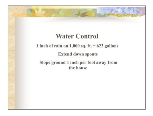
Approximately 625 gallons of water drains from the roof of a 1,000 sq. ft. house during a one-inch rain. Extend down spouts for several feet from the house, and slope the ground about 1 inch per foot away from the house to minimize the potential for roof water causing water problems in the home.
