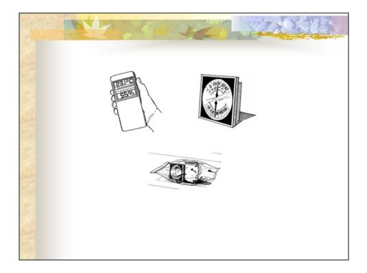
A hygrometer is used to measure relative humidity. A hygrometer needs to be calibrated to ensure accuracy. The hygrometer should read about 75% after being placed in a plastic bag with a cup containing about ½ cup of water and 1/4 cup of salt for a period of at least 12 hours. The hygrometer should be calibrated annually, since hygrometers tend to drift. Digital hygrometers tend to be more accurate.
