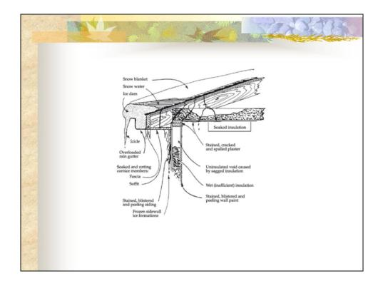
Problems associated with ice dams include staining of inside sheeting, wet ineffective insulation, rotting wood, and mold. Ice dams occur when the roof is warm enough to melt snow, due to heat from the house, while the roof over the soffit is cold enough to freeze the water.
