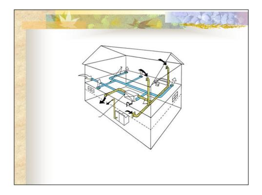
An air-to-air heat exchanger is an energy efficient method of obtaining the desired ventilation. Heat in the air being exhausted from the house is used to warm the air being brought into the house. A heat exchanger is about 70 - 80% efficient. A heat exchanger requires maintenance to be effective and efficient.
