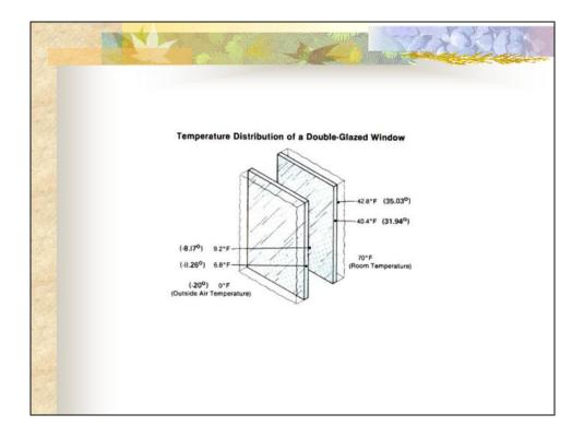
Due to condensation problems on windows, we cannot generally maintain humidity levels of 40% to 60% during the winter. When it is 0° F outside, the temperature on the inside glass surface of a double-glazed window will be about 43° F. When room air at 70° F and 40% relative humidity is cooled to 43° F at the window surface, the air relative humidity near the glass surface will be about 100% and condensation will be forming on the glass surface.
