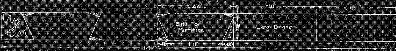
CUTS FOR ENDS, PARTITION, & LEG CROSSPIECES
