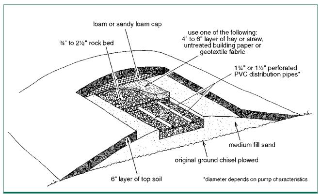
Figure 23. Construction features of a sewage mound.
