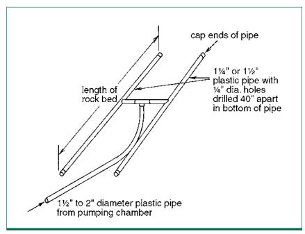
Figure 26. Pressure distribution system using two parallel pipes with a center feed. The pump in the pump chamber supplies effluent under pressure.
