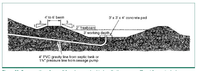
Figure 29. Cross section of a small farm lagoon sized to handle the sewage effluent from a typical three-bedroom home.
