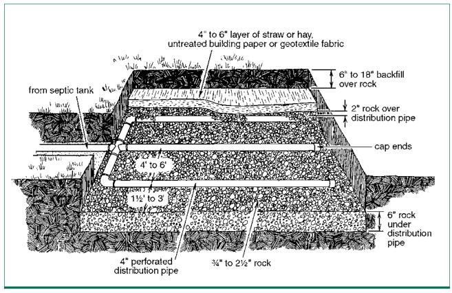
Figure 22. Absorption bed construction and layout.
