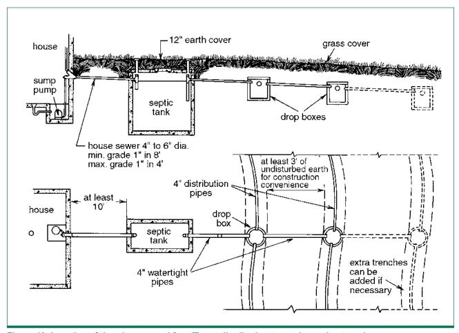
Figure 19. Location of drop boxes used for effluent distribution to an absorption trench system.
