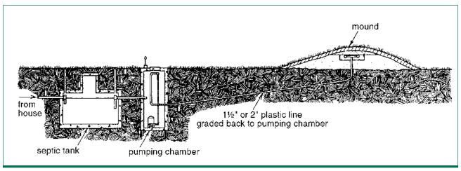
Figure 25. Septic tank, pumping chamber and sewage mound.
