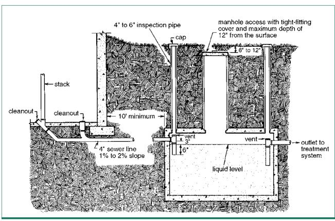
Figure 4. Deep septic tank installation. Suitable for use where a high water table is not present. Always check with the tank manufacturer to make sure the tank has the load- bearing capacity to handle the soil overburden.
