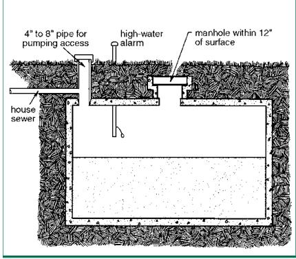
Figure 6. Holding tank for household effluent. Must be pumped on a periodic basis (usually every two weeks to a month).
