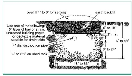
Figure 11. Cross section of a rock-filled absorption trench.
