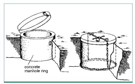
Figure 5. Methods of securing a manhole cover to prevent unauthorized entry.
