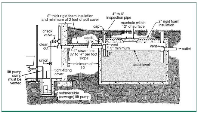
Figure 3. Shallow septic tank installation.
