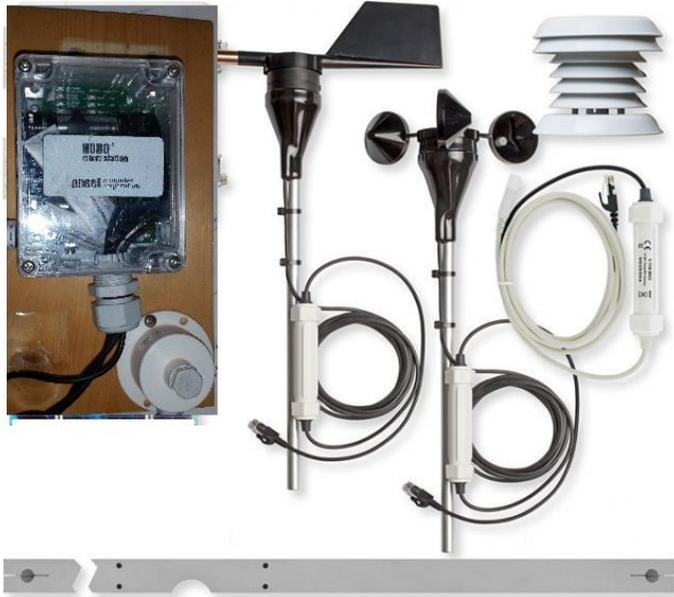
Figure 5. Onset Hobo Data Logger (H21-002) (Image partially from Onset Website – [www.onsetcomp.com](http://www.onsetcomp.com))
