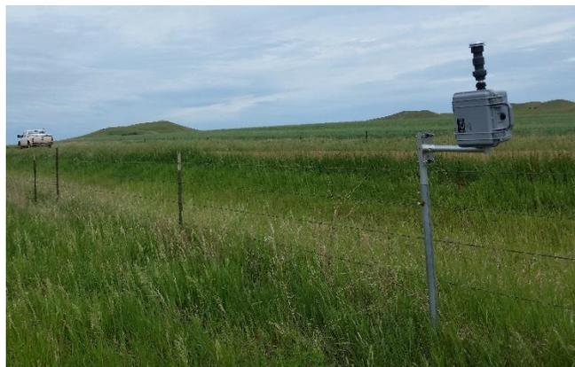
Figure 3. MiniVol™ Portable Air Sampler in operation at site #1 (vertically mounted)
