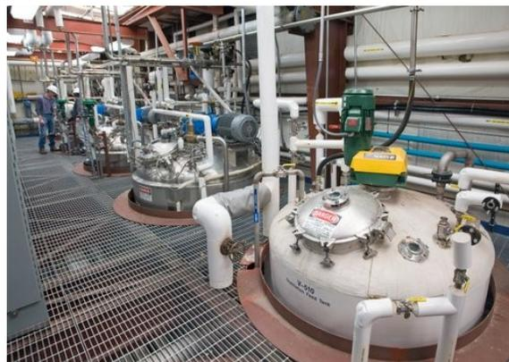
Ethanol fermentation tanks at the Biochemical Process Development Unit at the National Renewable Energy Laboratory's Alternative Fuels User Facility in Golden, CO. Photo by Pat Corkery, 2009. Courtesy of DOE/NREL.
