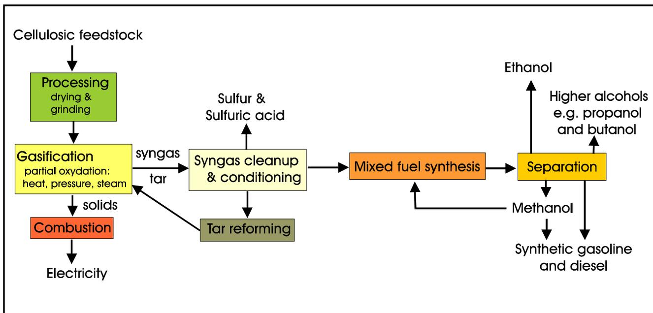
**Figure 3. Thermochemical production of cellulosic ethanol using gasification.**
