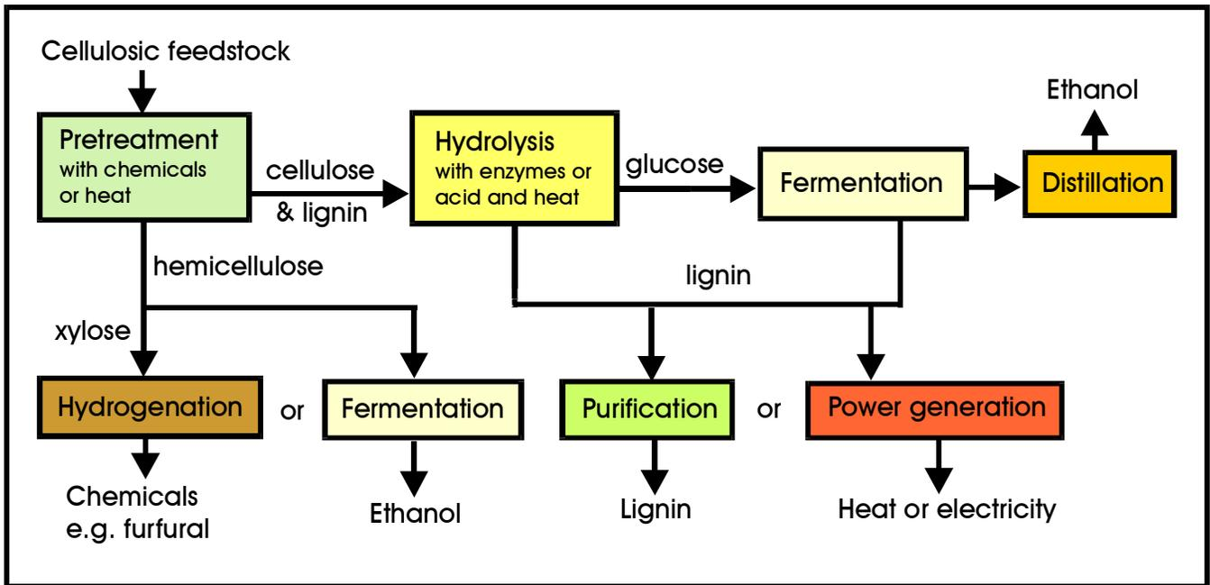
**Figure 1. Biochemical production of cellulosic ethanol.**
