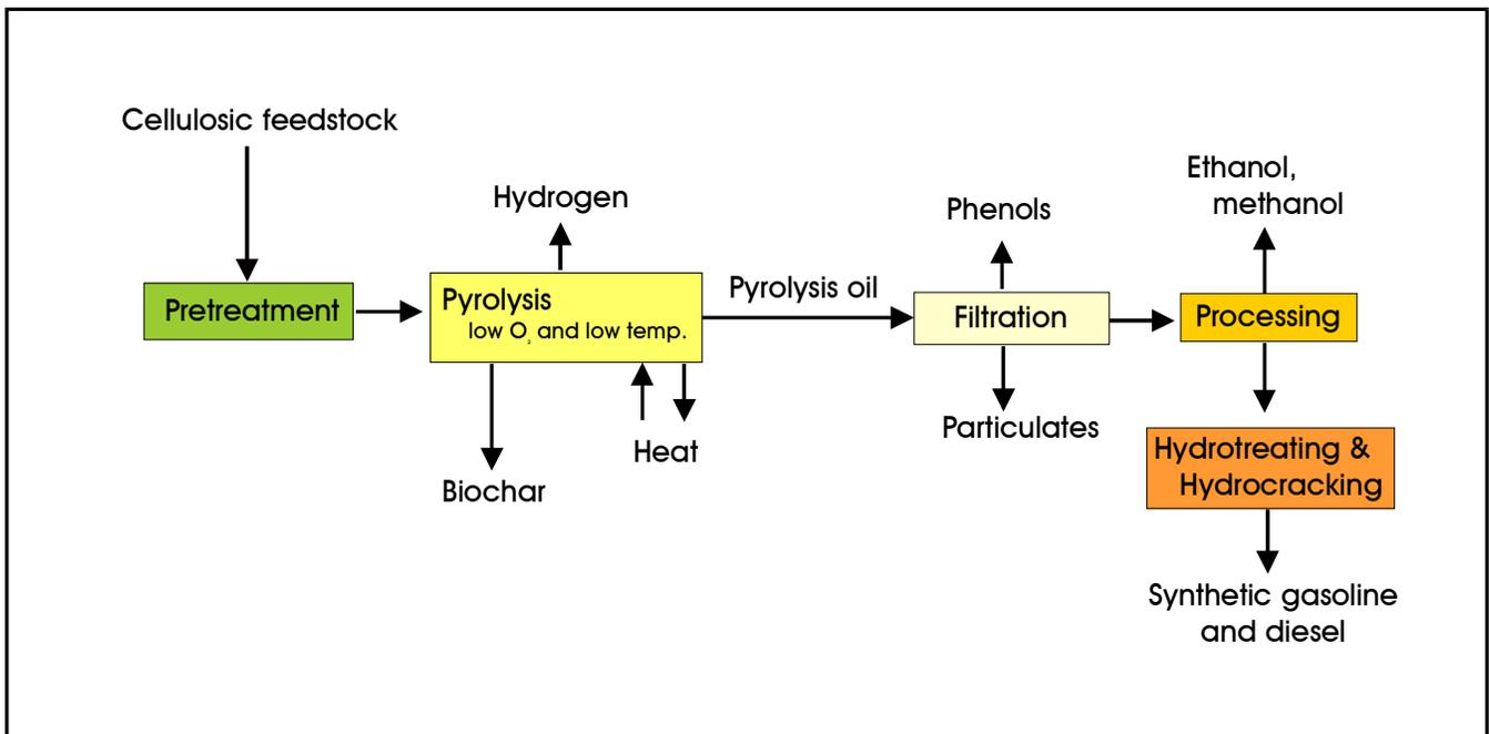
**Figure 2. Thermochemical production of cellulosic ethanol using pyrolysis.**
