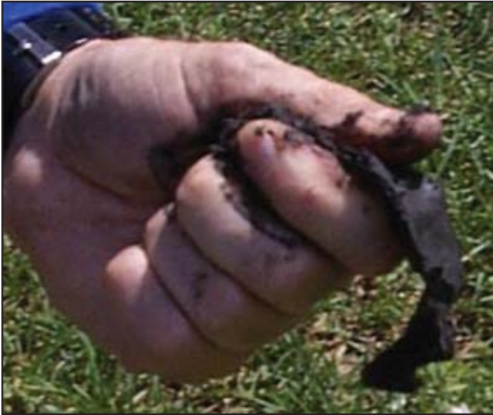
Figure 1. Determining clay content in soil via the ribbon test. This would be an example of a high-clay content soil.
