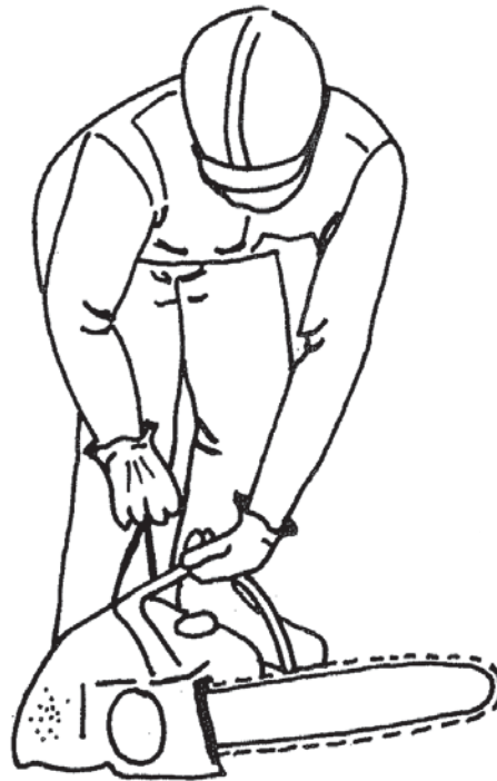
Figure 2. Start chain saw engine by setting saw on firm ground with chain out of gear and free of obstacles, placing right foot in loop of rear handle, pressing left hand down on upper handle and pulling starter rope straight up with right hand.
