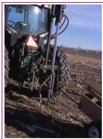
Soil sampling to the six foot depth
