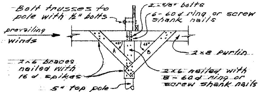
NOTE: short brace "A" should be located towards prevailing winds... west as shown in this drawing.
