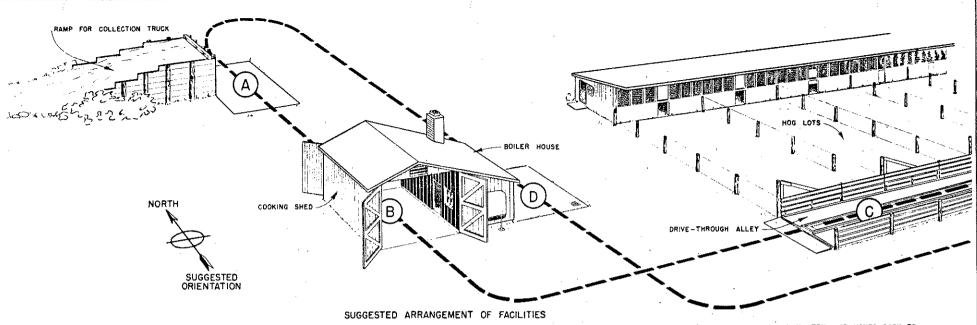
THE COLLECTION TRUCK' IS BACKED UP THE RAMP AND UNLOADED INTO THE COOKING TRUCK ON AN EASILY CLEANED CONCRETE PLATFORM. IT IS THEN WASHED AND MADE READY FOR ANOTHER COLLECTION.
